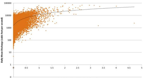
Figure 4 – Correlation of Antecedent Precipitation Index and Daily Mean Discharge (1949-present)
