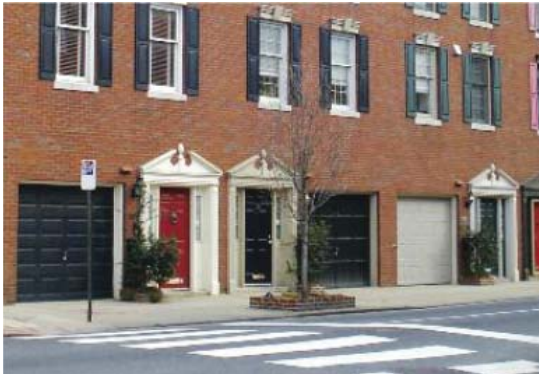
Many streets and homes in Philadelphia were not designed to accommodate driveways. Curb cuts can actually reduce overall parking capacity by eliminating on-street parking spaces. (Philadelphia Rowhouse Manual).
