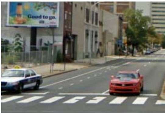
Wide vehicle travel lanes create additional impervious surface and may encourage higher vehicle speeds.
