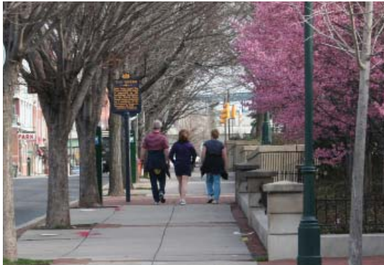
Two people walking side-by-side require 5’ of clear sidewalk space.
