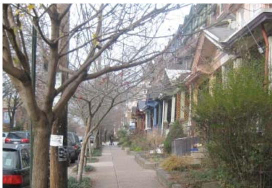
On Local Streets, minimum total sidewalk width is 10'.
