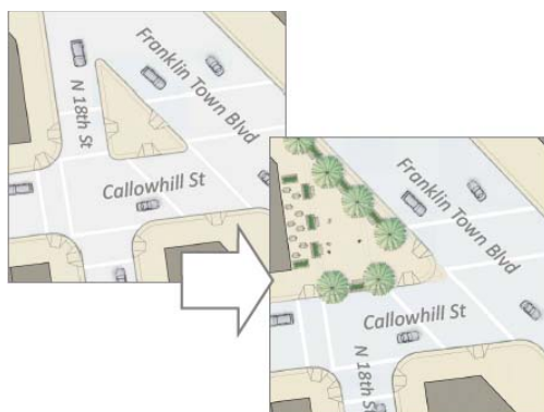
Complex intersections can be redesigned to eliminate conflict points and create an opportunity for public space and green infrastructure. (Adapted from San Francisco Better Streets Guide)
