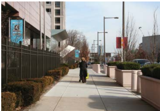
Planters should be located to maintain minimum walking zone widths (4.3.2).
