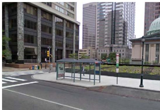
Curb extensions can be used at marked crossings to accommodate stormwater management features, street furniture, bike parking, transit stops, or other features. Above: John F. Kennedy Blvd and 18th St. Below: Queen Lane and McMichael St
