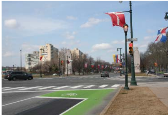
Bike Boxes can be combined with green colored pavement and “Wait Here” pavement markings to increase visibility.
