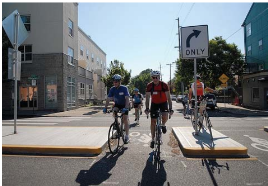
Diverters should limit motor vehicle movement, but enhance bicycle and pedestrian movement. (BikePortland)
