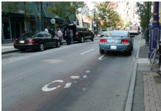
Outside lanes may be wider to accommodate buses, trucks, and bicycles.
