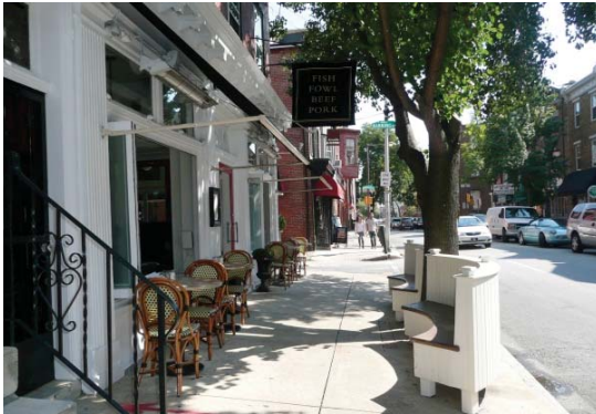
Sidewalk cafes (4.4.6) and other commercial activities on the sidewalk must maintain adequate clear width (4.3.2) for pedestrians.
