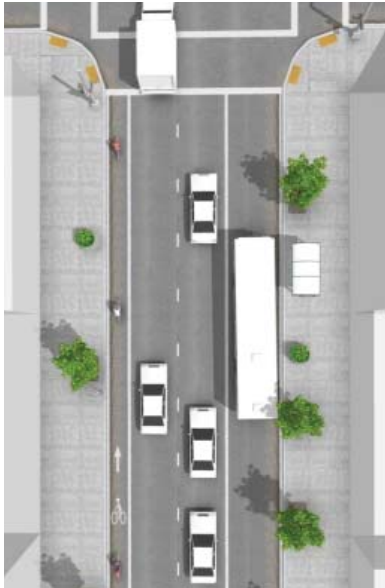
Typical left-side bike lane design (NACTO)
