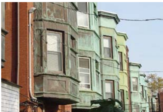
Bay windows may not extend onto or project over the minimum clear sidewalk width unless at least 10' vertical clearance is maintained.
