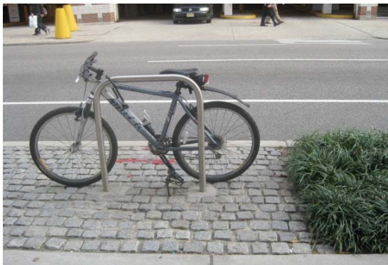
Different materials may be used to differentiate the furnishing zone and allow stormwater infiltration.
